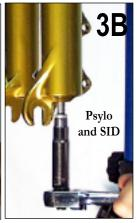
4. Tap the rebound shaft bolt and dual air shaft nut firmly with a plastic faced mallet to separate the shafts from the lower leg press-fit. Keep a bucket or oil pan below the fork to catch the oil. Inspect the condition of removed oil.
