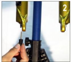
3. Using a 5 mm hex wrench, loosen the right damper shaft bolt five turns or halfway. Using a 10 mm socket, loosen the left shaft nut until it is flush or just beyond with the dual air shaft end.
