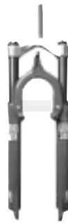
1995JudySL The fork that changed the world! 28mm upper tubes, easy to service cartridge design
